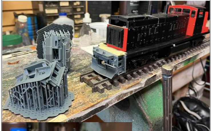
Left: Dan's loco with the 3D printed pilot (adjusted for large coupler)
