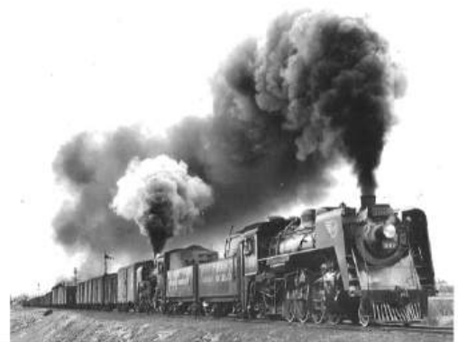
Vintage railway stations, Round houses, Locomotives, coaches, cabooses of Canada ... David Muma - January 6 at 8:17AM Twice the smoke An Ontario Northland Railway (ONT) double-header train Extra North, led by #307 and #311 2-8-0 Consolidations, leaving North Bay, ON in 1948. - source Hugues W. Bonin collection
